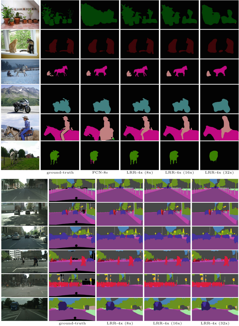
Fig. 11. Examples of semantic segmentation results on PASCAL VOC 2011 (top) and Cityscapes (bottom) validation images. For each row, we show the input image, ground-truth and the segmentation results of intermediate outputs of our LRR-4x model at the 32x, 16x and 8x layers. For the PASCAL dataset we also show segmentation results of FCN-8s [24].
