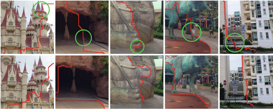
Fig. 6. Comparison of with and without our seam-guided local optimization. Top: Results without optimization. Bottom: Results with optimization.
