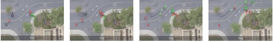
Fig. 4. Illustration of the class assignment for each target. The same color represents the same navigation style (cluster) described in Fig. 3. Note that for a given target its class changes across time regardless of its physical class ( i.e. , whether it is a pedestrian, bike, etc.). When the target is surrounded by other targets, its class changes with respect to its social sensitivity. In this scene, first we can observe a cyclist (shown as label 1 in the images) belonging to a black cluster, i.e. , being aggressive in his moves, then belonging to some milder clusters (purple and green). We also can see the evolution of a group of pedestrians (shown as labels 2,3) in the images), initially “mild” (green at T = 1 ), who become red at time T = 3 at which they decide to overtake another group and accelerate. (Color figure online)
