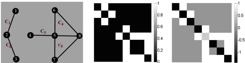
Fig. 2. An example graph (left), corresponding affinity matrix (middle), and scaled affinity matrix built considering vertex 5 as a user constraint (right). Notation C_i refers to the i^{th} maximal clique.
