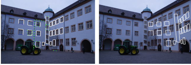
Fig. 1. Pose estimation results of OPnPL (left) and OPnP (right) in a scenario with a lack of reliable feature points. Blue points and solid line segments are detected in the image, and green dashed line segments are the model reference lines reprojected using the estimated pose. White lines are manually chosen on the 3D model to sketch its structure and projected onto the image to deem the quality of the estimated pose. Note also the shift along the line direction between the detected and the model lines. This issue needs to be handled in practice, where the reference lines in the model may only be partially detected on the image (due to partial occlusions). Images from [41].
