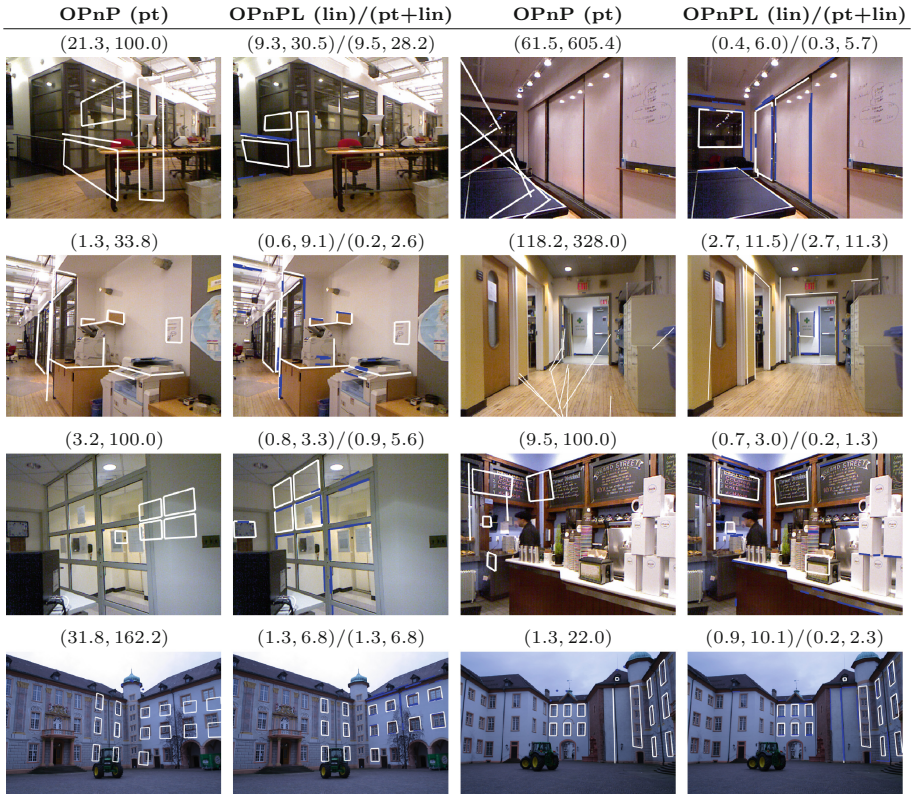
Fig. 8. Pose estimation on the NYU2 and Castle (last row) datasets, for OPnP and OPnPL. The numbers on top of each image indicate the rotation and translation error as pairs (Rot. Err. (deg), Translation Error (%)). For the OPnPL we report both the error of the only line case, and of the case with joint points and lines. The lines of the 3D model are reprojected onto the images using the estimated pose. For the OPnPL we reproject the lines using the pose estimated using both points and lines.
