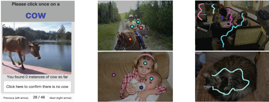
Fig. 3. Left. AMT annotation UI for point-level supervision. Center. Example points collected. Right. Example squiggles collected. Colors correspond to different classes. (Color figure online)
