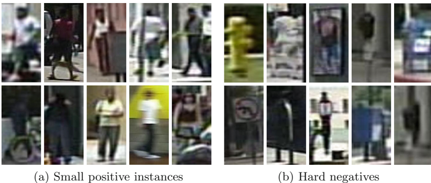
Fig. 1. Two challenges for Fast/Faster R-CNN in pedestrian detection. (a) Small objects that may fail RoI pooling on low-resolution feature maps. (b) Hard negative examples that receive no careful attention in Fast/Faster R-CNN.
