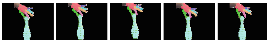
Fig. 8. Subset of tracked frames on the dataset of [38]. Our method can handle objects with varying sizes, colors, and different hand dimensions . Here we show how even a complex shape like a bowling pin can be approximated using only a few tens of Gaussians (Color figure online)
