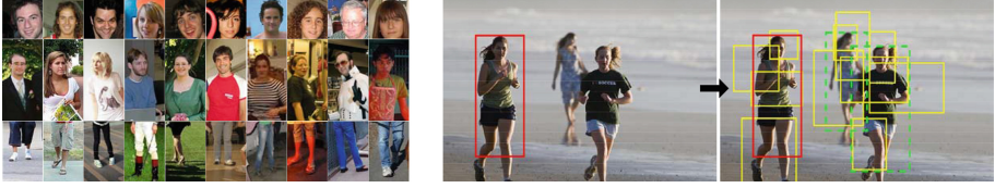
Fig. 3. Left: example poselet detections on the HAT [15] dataset. Right: example HAT image with only one bounding box annotation (red box) for a person. The yellow and green dashed boxes denote the detections of poselets and new people respectively. (Color figure online)
