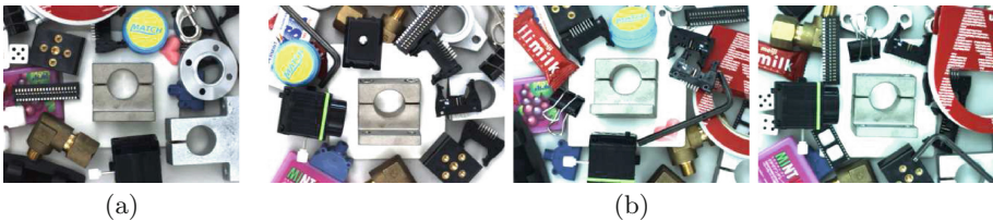
Fig. 5. (a) Vertical image and (b) three examples of perspective images for evaluation of the orientation features in experiment1. These images are almost identical except for the 3D pose of the target object (L-Holder at the center of the images).
