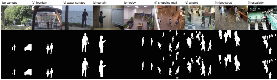
Fig. 3. i2R results: top row is the original image, second row is the ground truth, and the last row is our unrefined results without post-processing. We used the same frames as [15, 16, 22–25], for qualitative comparison.
