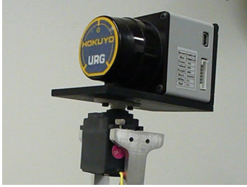
Fig. 5. First known design of 3D LRF with servo [10]
