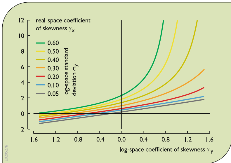
Fig. 6.6 Real-space coefficient of skewness \gamma_x for LP3 distributed X as a function of log-space standard deviation \sigma_Y and coefficient of skewness \gamma_Y where Y = \ln(X)
