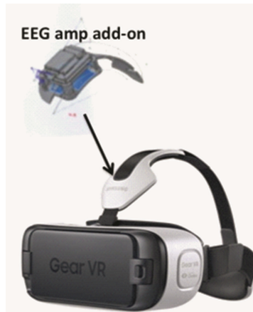
Fig. 4. UCSD Samsung Gear VR goggle adapted with integrated EEG sensing technology and eye movement system [7].
