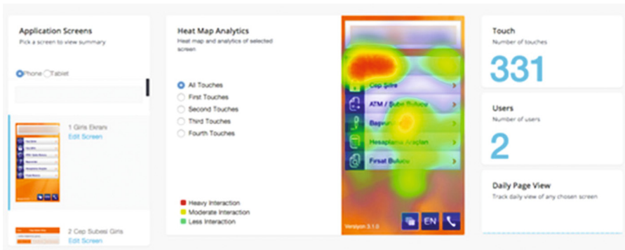
Fig. 2. Head map feature for tracking user operations on a mobile app (Image Source: AppAnalytics.io).
