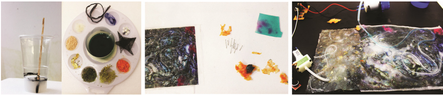
Fig. 2. Left: Silicon Mixture and ingredients [colored powder, gold-flakes, grass fibers, beads, yarns]. Middle: Multilayer making process. Right: Multi-layer composite with active texture and fluid actuation. (Color figure online)
