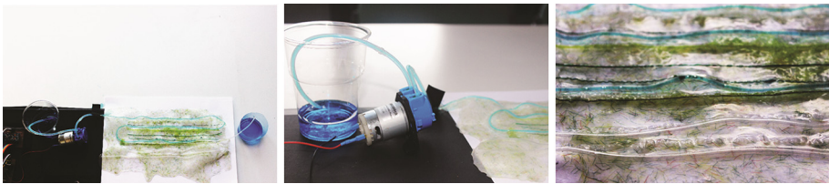
Fig. 4. Tests on sound-activated fluid-actuation layer. Composite embedded with grass fibres and silicon tubing.
