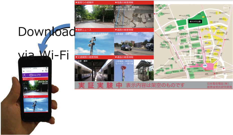
Fig. 4. Signage-smartphone collaboration. Evacuees can download a map or route to the nearest evacuation center via local Wi-Fi.
