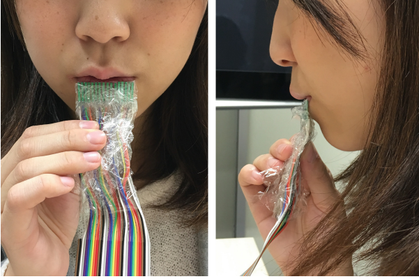
Fig. 1. This picture shows how to use the stimulation unit. Users apply the stimulation unit on one’s lips by having it in one’s hand. In this paper, they apply it on lower lip only.
