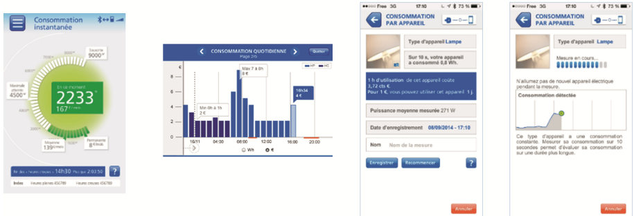
Fig. 1. (from left to right) Start screen showing instantaneous power and consumption, graphical history (daily consumption), consumption information per appliance (measurement underway), consumption results per appliance.
