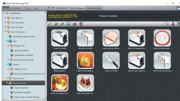
Fig. 1. AssisT-Task authoring tool. In the example the "Make toasts" tasks is shown
