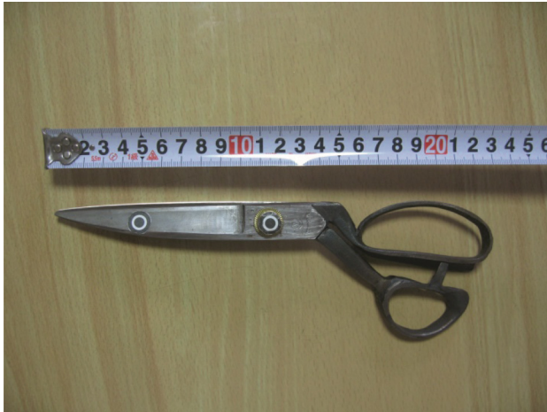
Fig. 1. Pairs of so-hizukuri forged scissors (The length of the blade: Thumb finger ring side 99.0 mm, Other four fingers side 100.0 mm).
