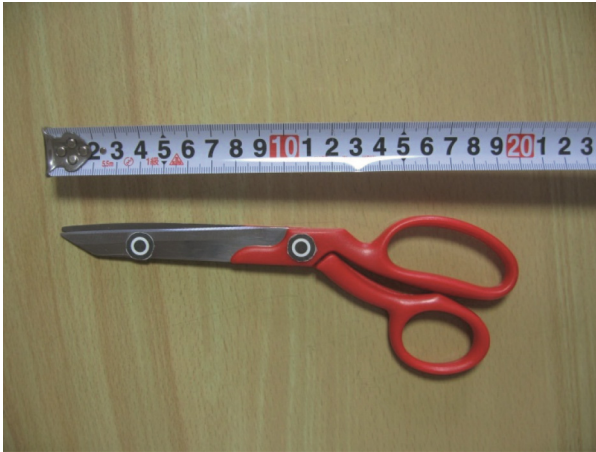
Fig. 2. Pairs of purchased from a 100-yen shop scissors (The length of the blade: Thumb finger ring side 85.0 mm, Other four fingers side 99.0 mm).
