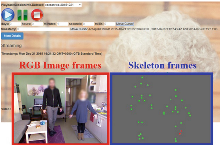
Fig. 3. The CAC Playback Manager Web App ( http://www.cac-framework.com/app ). Skeletons streaming (Right) and RGB Video streaming (Left) are handled by the integrated CAC client.
