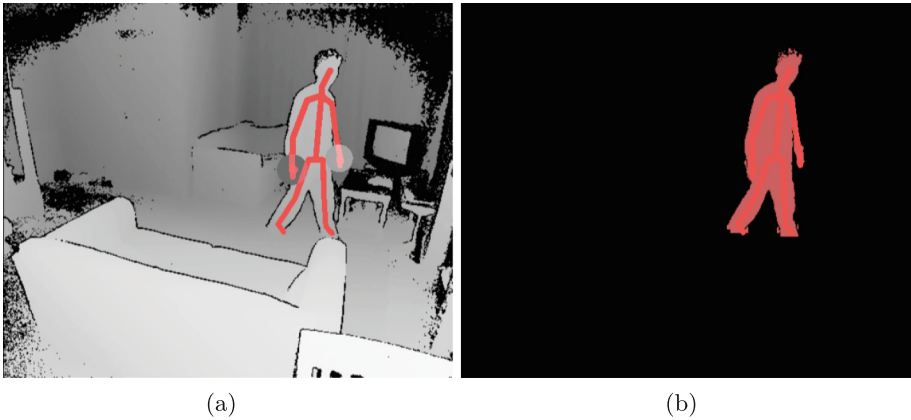
Fig. 4. Kinect sensor installed in a residential setting. (a) The background is subtracted while depth silhouettes and skeletons are determined by the Kinect SDK. (b) Infra-red and depth sensing from the similar image.
