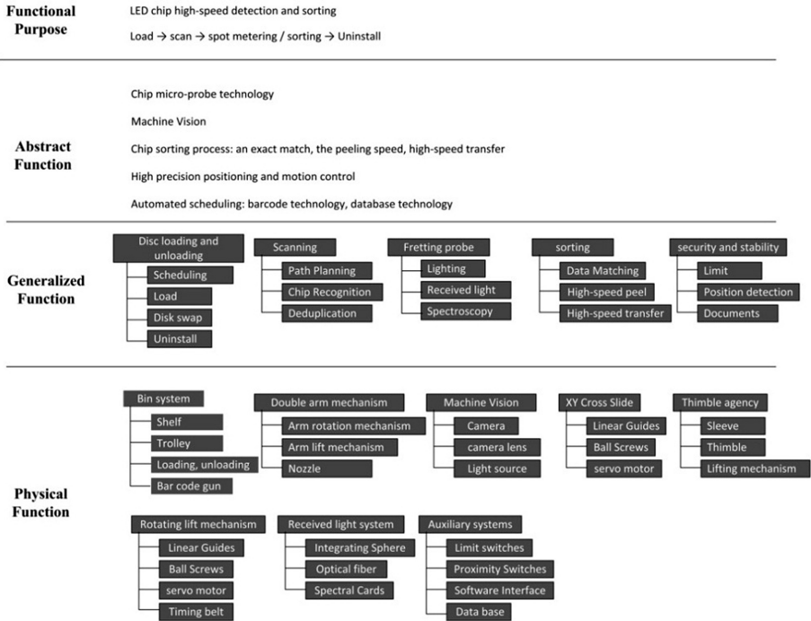
Fig. 6. Work domain model in LED chip high-speed detection and sorting system
