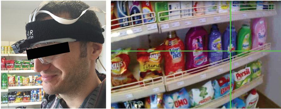
Fig. 3. A participant wearing the fNIR sensor as well as the ASL mobile eye tracker (left). A grocery store setup was used to investigate purchasing decisions in a more ecologically valid shopping scenario.
