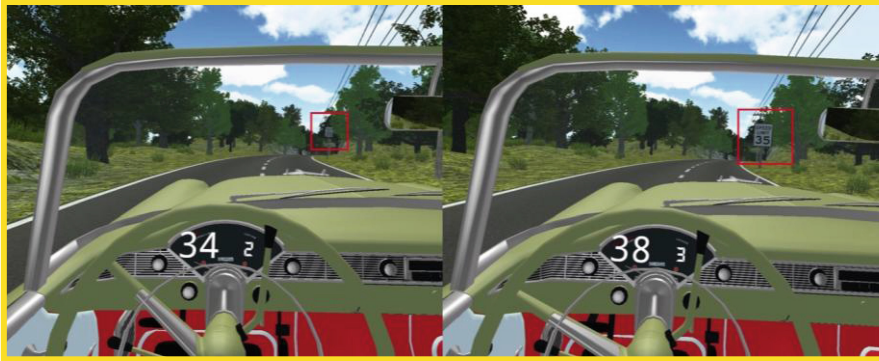
Fig. 3. An example of a possible compensatory augmentation. Left image has a normal size sign while the right image shows a sign that has been enlarged as the driver approaches.
