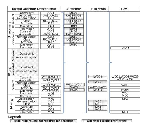
Fig. 3. Selection process of the mutation operators used for evaluating testing approaches
