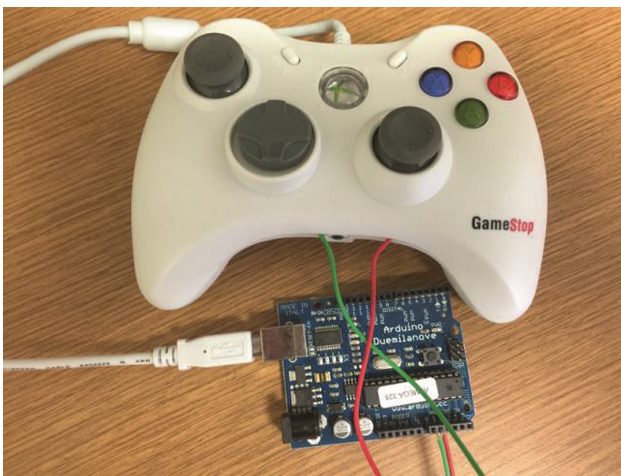
Fig. 2. Complete haptic capture controller modification with arduino board
