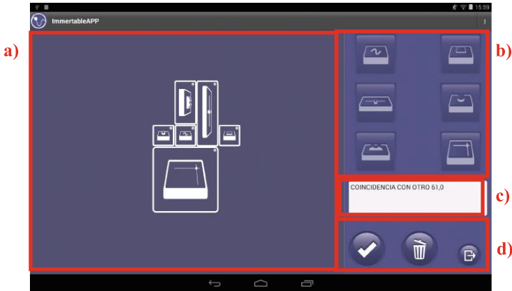
Fig. 2. Graphic editor interface: (a) Work area, that will be visualized later in the tabletop surface, (b) Controllers area, that can be included in the work area dragging and dropping them, (c) Feedback and user information area, and (d) menu area.
