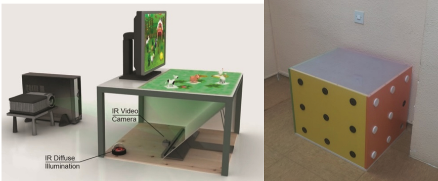
Fig. 3. Left: NIKVision tabletop [5]. Right: ImmertableApp tabletop (no monitor, it has a picoprojector inside it, it is more robust and with colors for children).
