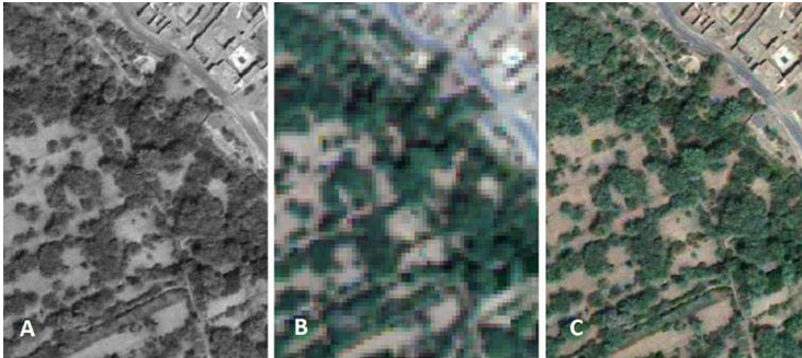
Fig. 3. Fusion process (C) of multi-spectral bands (B) with panchromatic band (A)
