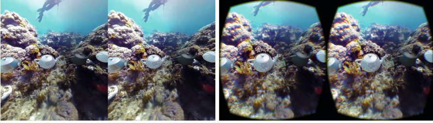
Fig. 1. IBL rendering for stereoscopic output using 360^\circ video via our pipeline (left), and the result in head-mounted display (right).
