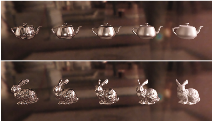
Fig. 6. Glossy specular reflection for various lobe sizes determined by a roughness parameter of, from left to right: 0.01, 0.05, 0.1, 0.2, 0.5.
