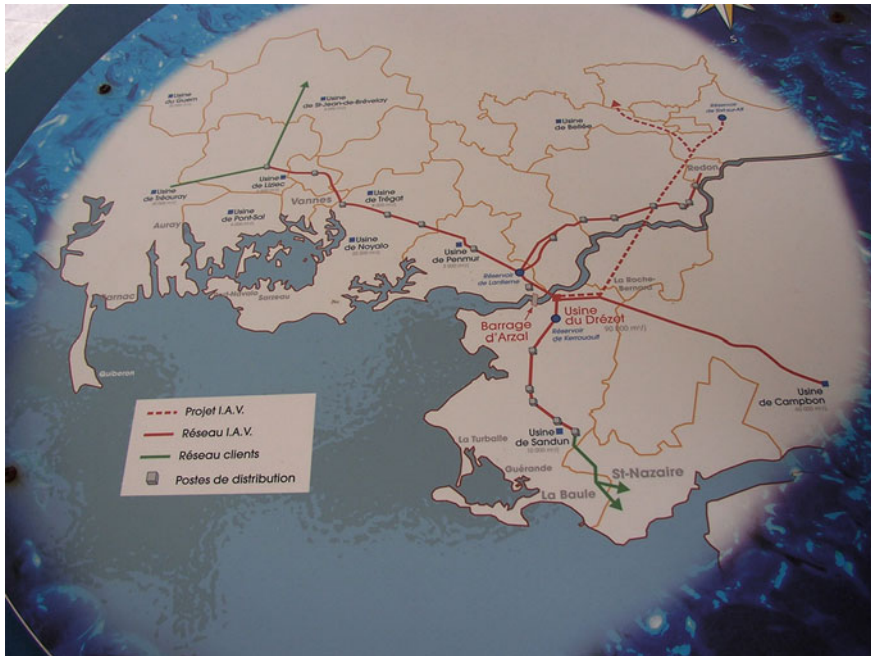
Fig. 11.2 Drinking water provision network of the Vilaine catchment and connections. Map displayed at the Drézét water plant. Photo Isabelle La Jeunesse, 16/09/2013
