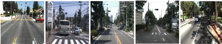
Fig. 1. An illustration of the various challenges in the lane detection including the absence of lane markers, degraded lane markers, shadows and occlusions.
