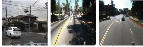
Fig. 5. Missed lane marker detections by our algorithm, for a hard left turn and suddenly emerging left lanes.
