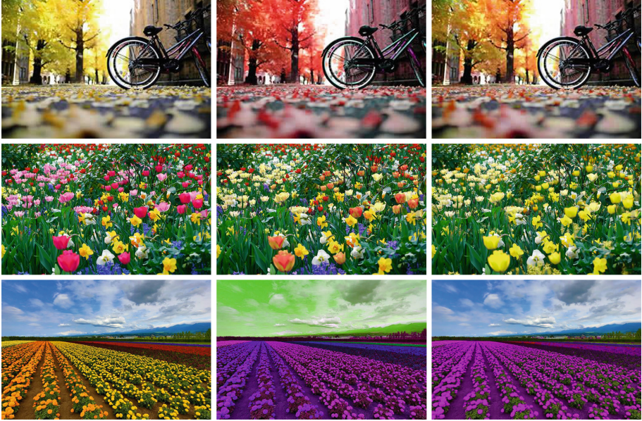
Fig. 13. Examples of hue transfer compared to Photoshop. Row 1 shows the results after hue stretch. Row 2 shows the results after hue compression. Row 3 shows the result after hue shift.
