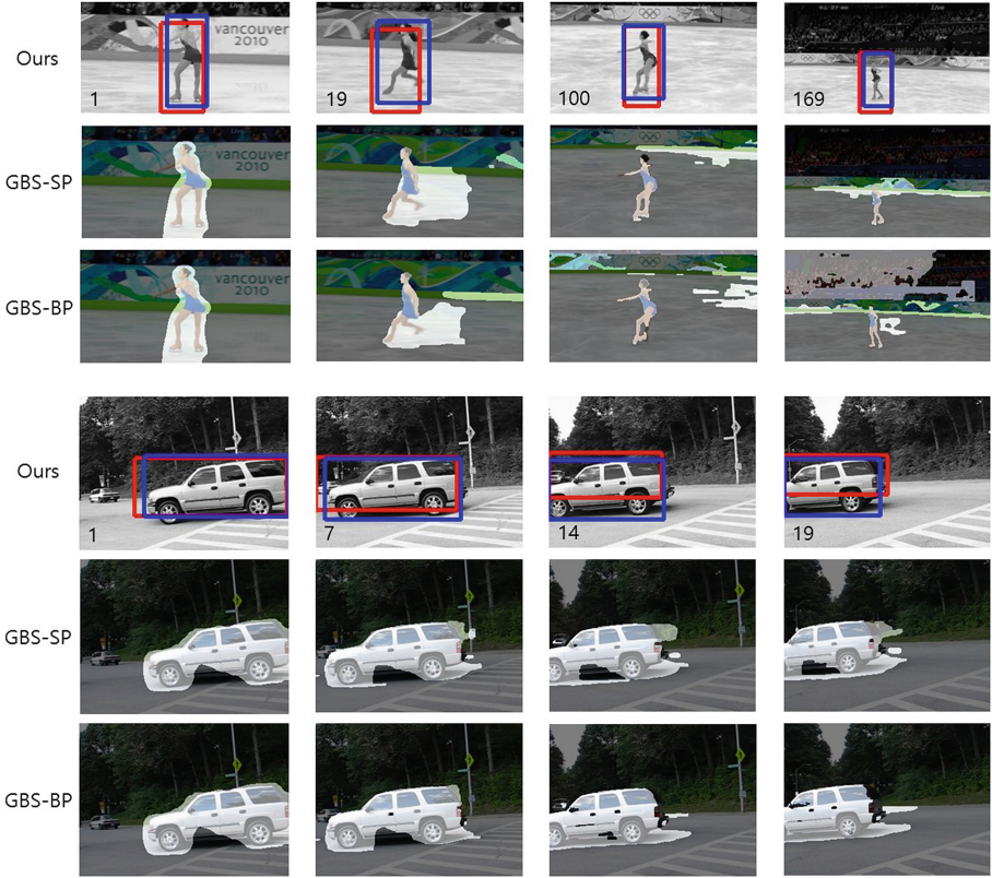
Fig. 3. Comparison with the proposed algorithm, GBS-SP, and GBS-BP for skating video with inexact initial label. The images in each column represents the tracking result of each algorithm. The blue box represents the ground truth bounding box and the red box represents the tracked bounding box. Notice that the foreground label of GBS-SP and GBS-BP are spread out over time (Color figure online).
