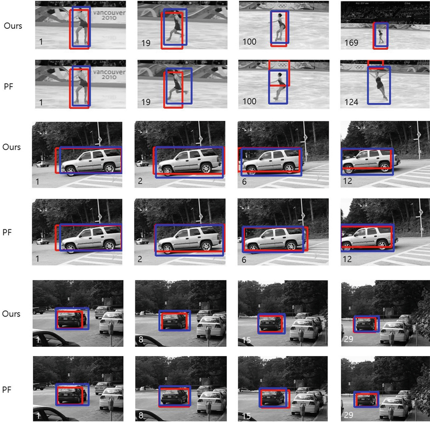
Fig. 2. Comparison with the proposed algorithm and particle filter for skating , car1 and car2 video. The images in each column represents the tracking result of each algorithm. The blue box represents the ground truth bounding box and the red box represents the tracked bounding box. Notice that the particle filter can not follow the foreground object in skating video (Color figure online).
