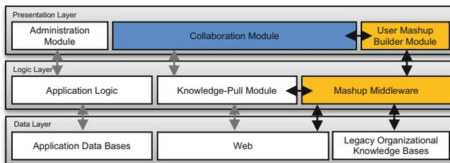
Fig. 2. Simplified high-level architecture of the software tool
