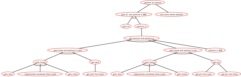
Fig. 6. Attack tree generated by the prototype implementation for the example shown in Figure 1.
