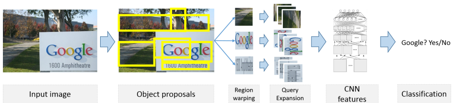
Fig. 1. Outline of the recognition pipeline: (1) Candidate objects regions are extracted from the image. (2) Regions are warped to a common size and multiplied through Query Expansion. (3) CNN features are computed over each region. (4) Classification is performed using linear SVMs.
