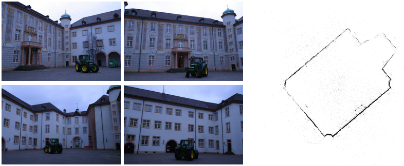
Fig. 1. Left: sample images of the Castle-P30 dataset. Right: sparse 3D reconstruction obtained with our pipeline. The root-mean-squared reprojection error (RMSE) is 0.1681 pixels.
