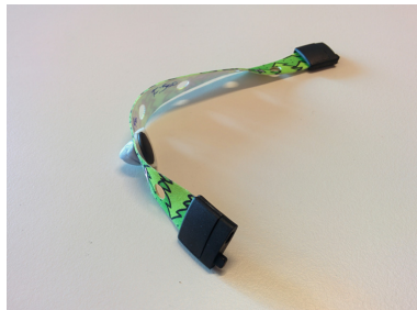
Fig. 2. Original prototype bracelet with an NFC tag embedded in a widget
