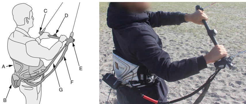
Fig. 5. (Left) Elements of prototype: (A) harness, (B) microcontroller enclosure, (C) left vibrotactile actuator, (D) accelerometer and center vibrotactile actuator, (E) right vibrotactile actuator, (G) safety leash, (F) signal wire. (Right) Control bar prototype in use during study session.
