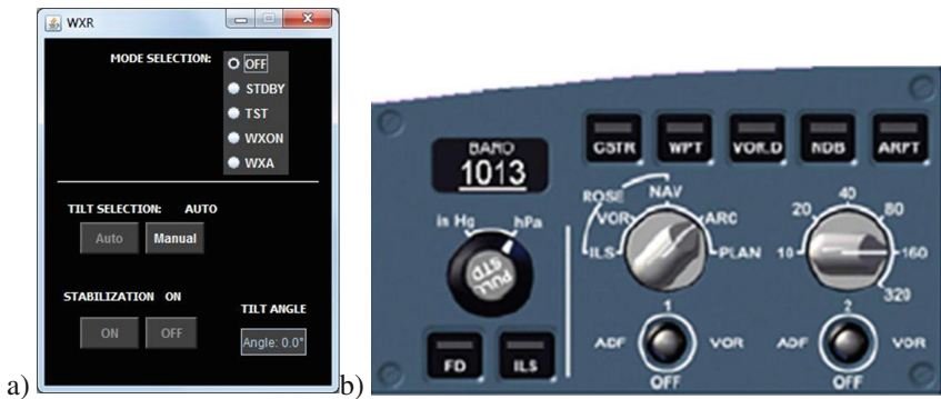
Fig. 3. Image of (a) the numeric part of weather radar control panel (b) physical manipulation of the range of the weather radar
