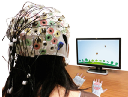
Fig. 1. A participant receives tactile feedback while controlling the MI-BCI. Vibrations from the motor on the right hand represent the current feedback provided by the MI-BCI system.
