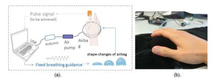
Fig. 2. (a). Touch Airbag schematic diagram. (b). The user's right hand on the airbag
