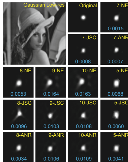
Fig. 1. An illustrative example of the bi- \ell_0 - \ell_2 -norm regularization for nonparametric blur-kernel estimation in single image blind SR. This figure shows the two times interpolated low-res image Lena (Nearest Neighbor), the ground truth blur-kernel, and the estimated ones using regularizations (7)-(10) with NE, JSC, ANR for generating the reference image \hat{\mathbf{u}} . The parts denoted by 5-NE/JSC/ANR correspond to the full scheme without continuation.
