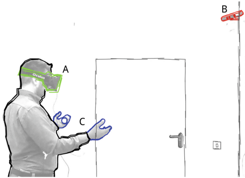
Fig. 1. Setup for the experiment. The virtual training environment is displayed using an Oculus Rift (A). The user is tracked by a Kinect (B). Opening and closing of hands is detected by gloves (C).
