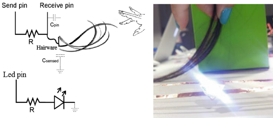
Fig. 3. Hairware as a capacitive sensor. (a) Circuit of Hairware as an input device. (b) Touching Hairware to trigger LEDs.
