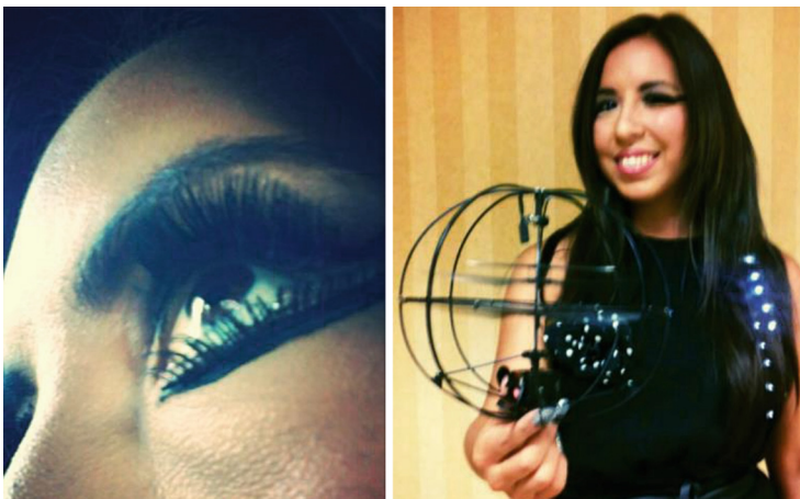
Fig. 1. Conductive makeup. (a) Conductive eyelashes and eyeliner in natural coloration. (b) Superhero project that levitates a drone by blinking.
