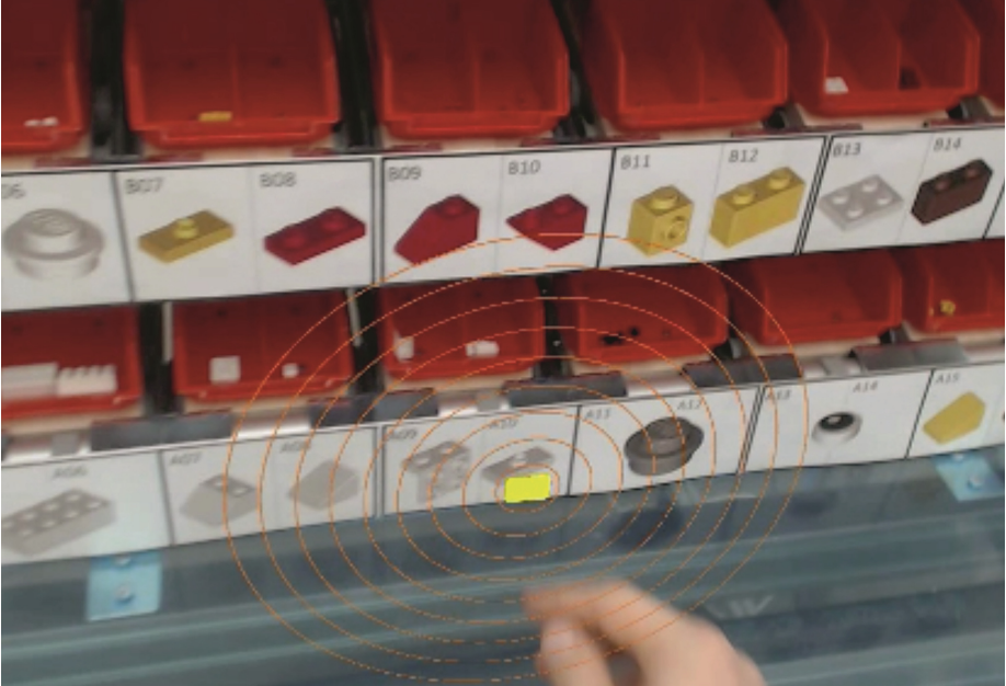
Fig. 3. Picking support based on the augmented reality technology: the object of interest is visually highlighted in the user's field of view
