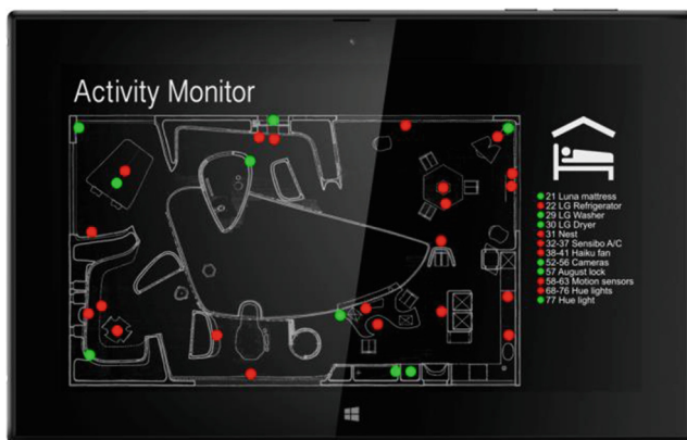
Fig. 5. Activity View: This view monitors specific living activities throughout the house by showing simple on/off functions of specific devices linked to the selected activity. For example for a sleeping activity the refrigerator goes into away mode, the washer and dryer start their operation, A/C units are shut down, along with lights, motion sensors and the door is locked.
