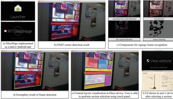
Fig. 4. We developed a mobile app, namely GlassNage , to perform the following functions: (1) layout recognition from an image captured using camera equipped device, (2) perform perspective correction, (3) let a user selects a section which s/he wants to receive further information from, and (4) visualize a website containing content's detailed information. We describe our layout recognition approach in (b)–(e).
